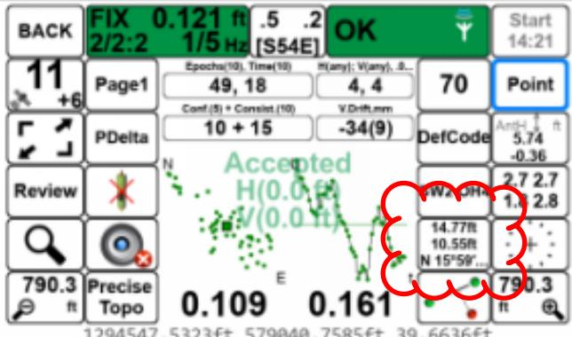
The distance between 69 and 70 was only 5 feet horizontally in field. Point 70 was out Horizontally 8' in a SW direction and 10' vertically.
