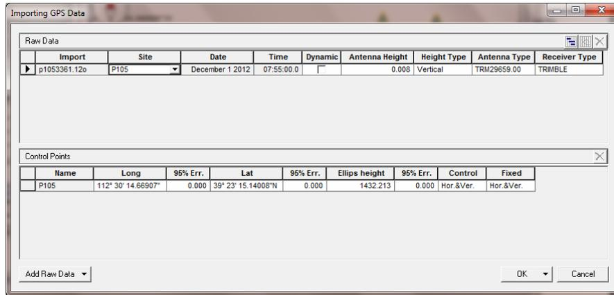
Take a moment do to a reality check on the antenna height, the height type and antenna type. Sometimes GNSS Solutions will not be able to match the antenna type / dome information from the RINEX file and the internal antenna database. When this happens, the 'Antenna Type' value will be bold highlighted and you will need to manually match up the correct antenna.
