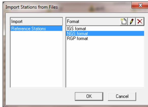
and then click on ‘OK’. Browse for the file containing both computed and HTDP stations, make sure the “Terrestrial Reference” is set to “WGS84” (yes I know this is wrong—it is part of the hotwiring, just go with it for now) and don’t worry about the default epoch as it is set on each entry in the station list:
