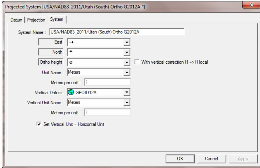
Choose 'GEOID12A' for the 'Vertical Datum', change the 'System Name' to something appropriate; I used "USA/NAD83\_2011/Utah (South) Ortho G2012A" for Utah South.
