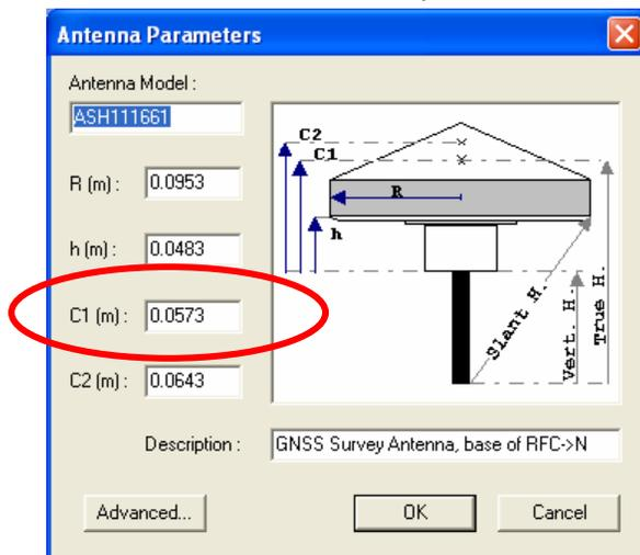
If C1 is 0.0573 then you have successfully loaded absolute calibration values. If C1 is 0.0754 then you screwed up and still have relative antenna values.
