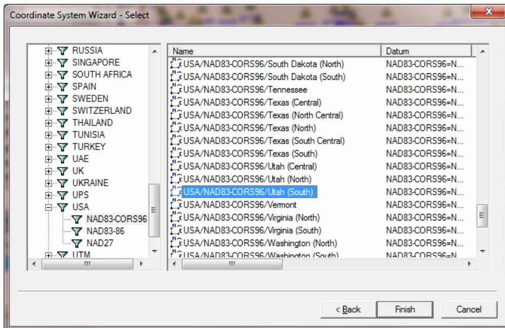
Double-click on the new state plane system (USA/NAD83-CORS96/Utah (South) in this case) to edit the configuration:
