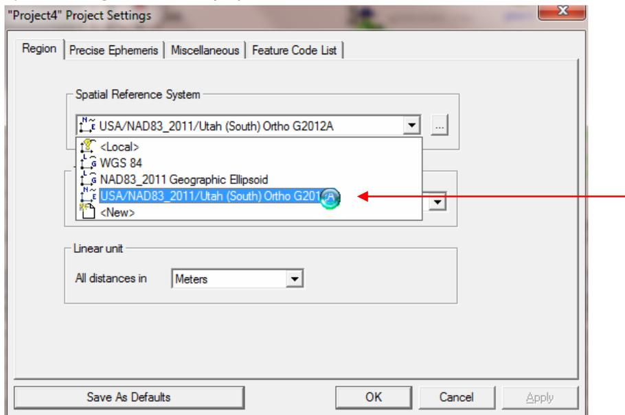
Drop down the ‘Spatial Reference System’ combo box and choose the state plane projection we setup earlier. Press OK.
