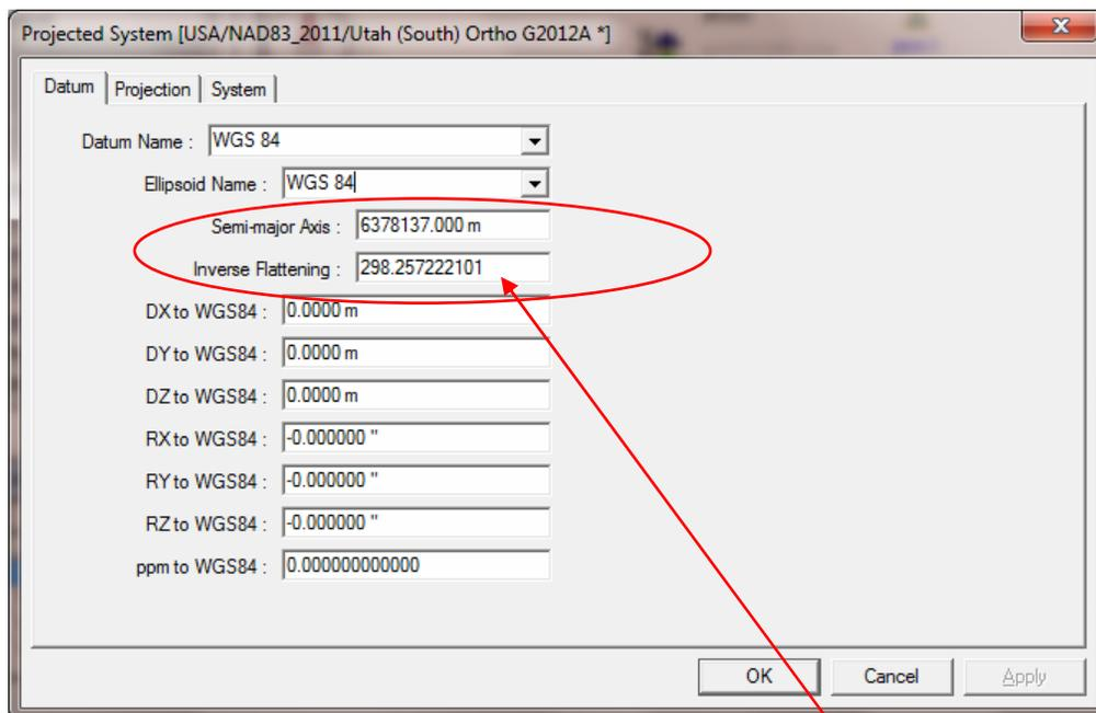
**This is IMPORTANT:** Change the 'Datum Name' to 'WGS84'; make sure the 'Ellipsoid Name' is 'WGS84' and most importantly make sure the "Inverse Flattening Ratio" is **298.257222101** as shown above. (More hotwiring here, just go with it for now.)
