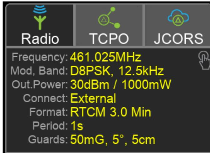
Tapping this box opens the *Base Configuration* screen. The options you wish to use need to be checked. Multiple correction stream sources can now be selected. You can have your base broadcasting both through a radio and through TCP or JCORS.
