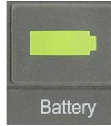
When the **TRIUMPH-LS** is turned on and not charging, the upper right and lower left LEDs give you a quick indication as to the status of the two battery packs. For more detailed information regarding the status of the two battery packs as well as other internal conditions and behaviors during the previous 30 hours, tap on the battery icon. or give the battery key a push
