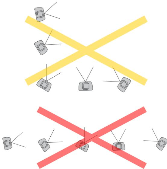
◆ In addition to the points of the object being investigated (target), it is necessary to provide a sufficient number of tie points. It will be perfect to have 4-5 points visible on all images. If it is unachievable, it is necessary that on each image there are minimum 3 common points, visible at least on three shots each. The minimum condition for obtaining solutions is to have on every shot three points each visible on at least one shot more.
