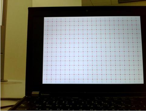
And following is an example of bad photo – note the clearly visible reflection of some of calibration pattern dots in the glossy laptop case:
